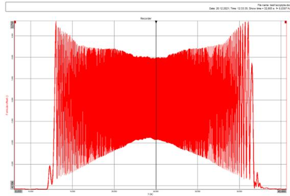
Fig. 5. Time courses of the recorded excitation plate displacements
