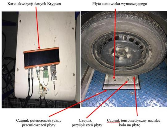
Fig. 2. Test vehicle on the test stand and elements of the measurement system
