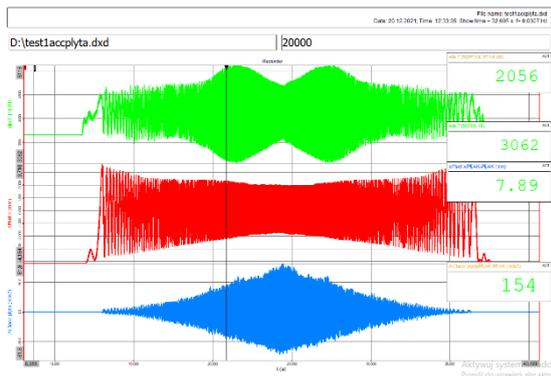
Fig. 3. Time courses of the signals recorded for the vibration test (dynamic load, plate displacement, plate acceleration)
