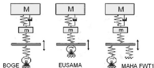
Fig. 1. Kinematic diagrams of the methods engaged to induce plate vibrations in shock absorber testing stands by the forced vibration method [8]
