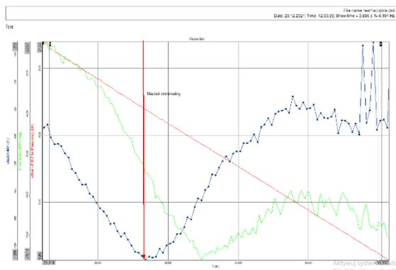
Fig. 9. Frequency change profile: excitation – red; envelope of the wheel load on the test stand plate – blue; phase angle change profile for displacement and force signals – green
